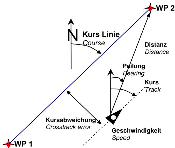
**Caution:** Track or Tracklog is also called the sequence of recorded positions during one flight.
