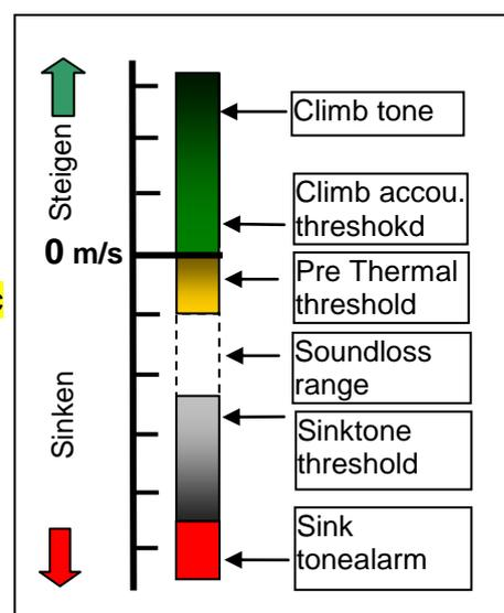
**Sink Alarm** =Sink alarm threshold
