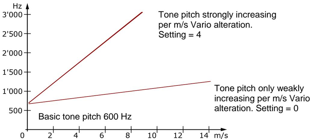
**2.2.6.4 Variometer Climb acoustic → Pitch change / increase of tone interval per m/s**
