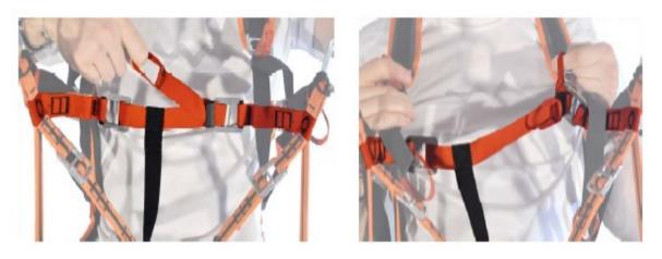
Each setting the harness must be done with mounted protector, rescue system and be symmetrical on both sides.
